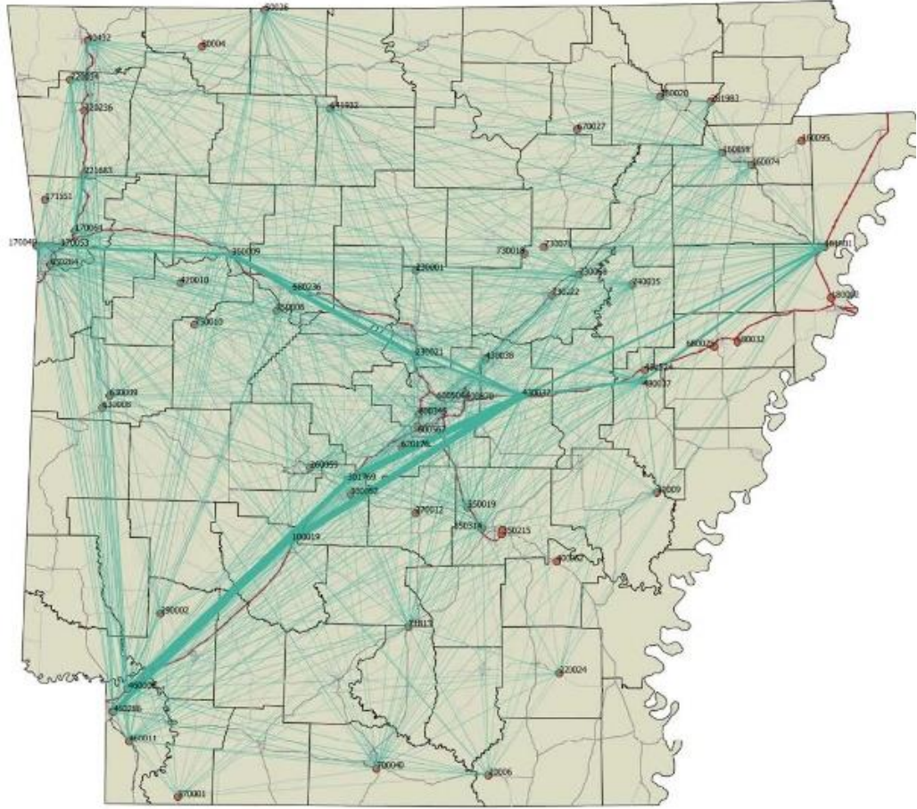
Figure 13. Connectivity of WIM Sites by Individual Trucks Subscribing to Drivewyze (Open Source Image).
